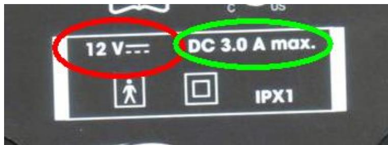
The part of the symbol with the solid line above the dashed line is the international symbol for DC voltage.
