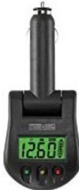
A fully charged lead-acid battery with no load will read somewhere in the 12.8v range or higher. A lead-acid battery is considered completely discharged when the meter reads 12.0 volts. Pulling more energy out of a fully-discharged lead acid battery will cause internal damage, eventually destroying the battery's ability to hold a charge. Plan on recharging when you hit 12.2 volts.
